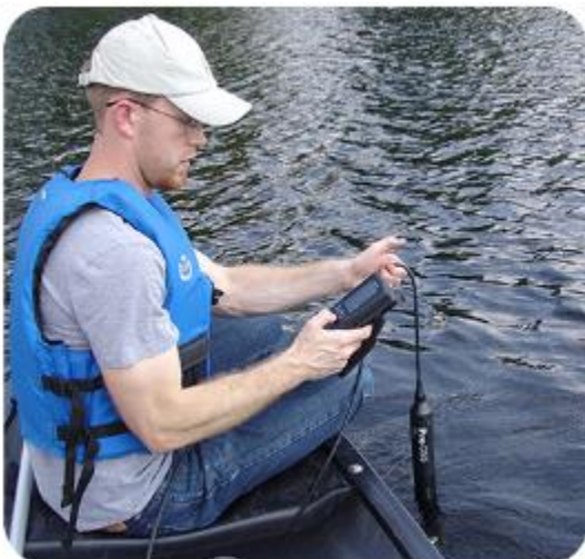
Figure 15: A scientist assessing water quality using a YSI instrument (Geotech Environmental Equipment 2020)
